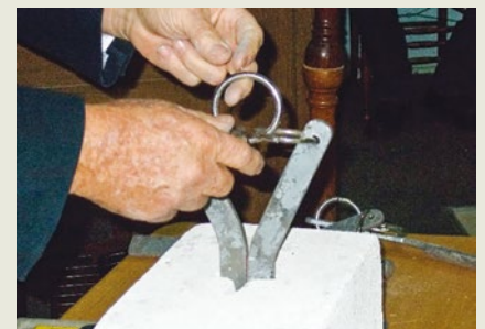
A demonstration of a stone lewis
